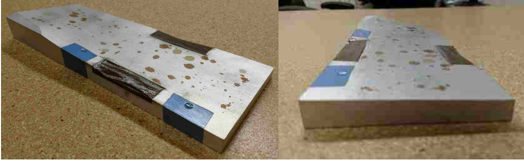
Figure 6.4: Aluminum plate used to tool the blade spars, twisted to follow the blade chord profile.
