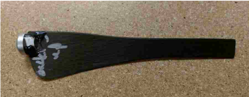
Figure 6.5: Blade spar with aluminum hub connection.
