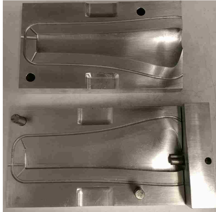
Figure 6.6: Aluminum mold used to cast the urethane around the blade spar.
